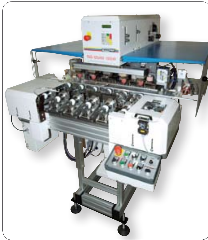
TSG 200/150-210/41 Special design - Precision multi-colour print on golf balls
