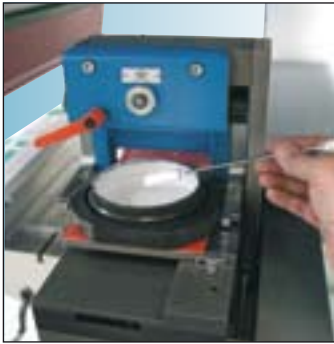
Checking of the ink without dismounting the ink/doctoring cup
