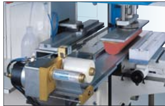
Tampon cleaning systems ("TSQ 60" & "TSQ 90")
