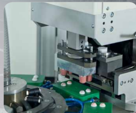
Automation with 4-fold use 36.000 parts/h
