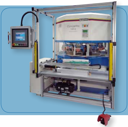
Semi-automatic machine for washing machine panels
