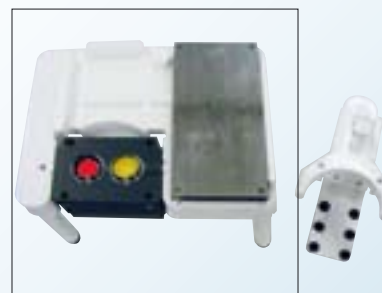
Multi-colour thrust ring for 2-colour printing
