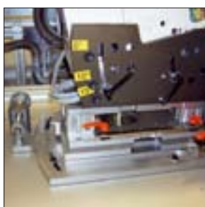
Cross table with inclination adjustment
