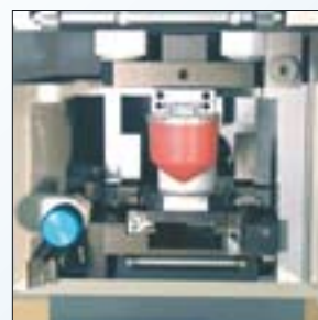
Cliché holder with Ø 60 mm ink/doctoring cup (retrofitted)
